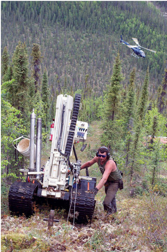
A worker moves a GT Probe rock and soil sampling machine on White Gold's property in the Yukon. Credit: White Gold.
