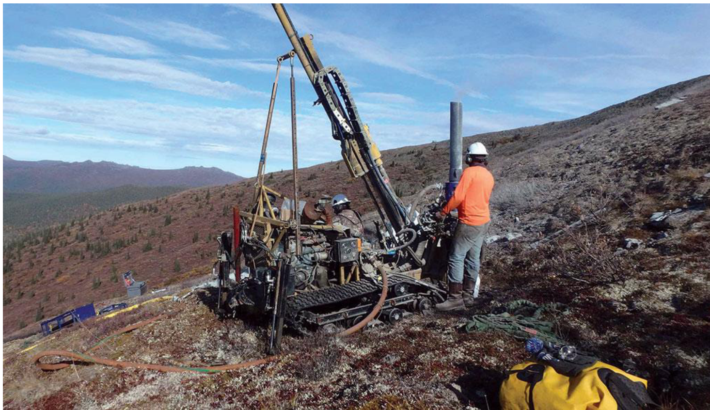
Rotary air-blast drillers on White Gold's Betty gold target in the Yukon. Credit: White Gold.
