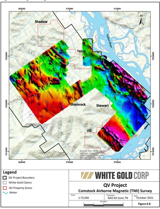
Figure 6.8: Comstock airborne Magnetic (TMI) survey
