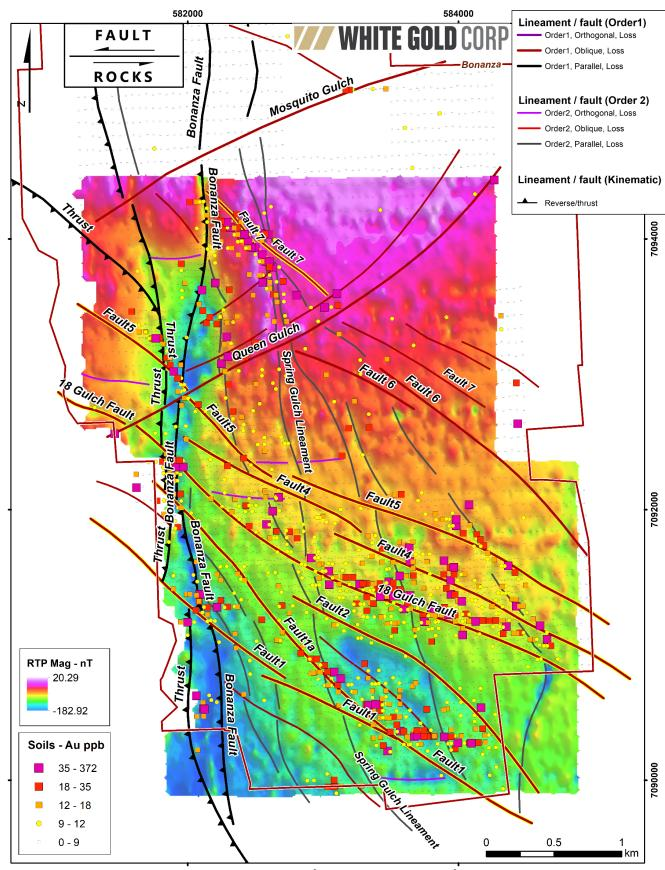
Figure 5: Interpreted Structures (Fault Rocks Inc.) and Gold in Soils on RTP Magnetics Base Map.
