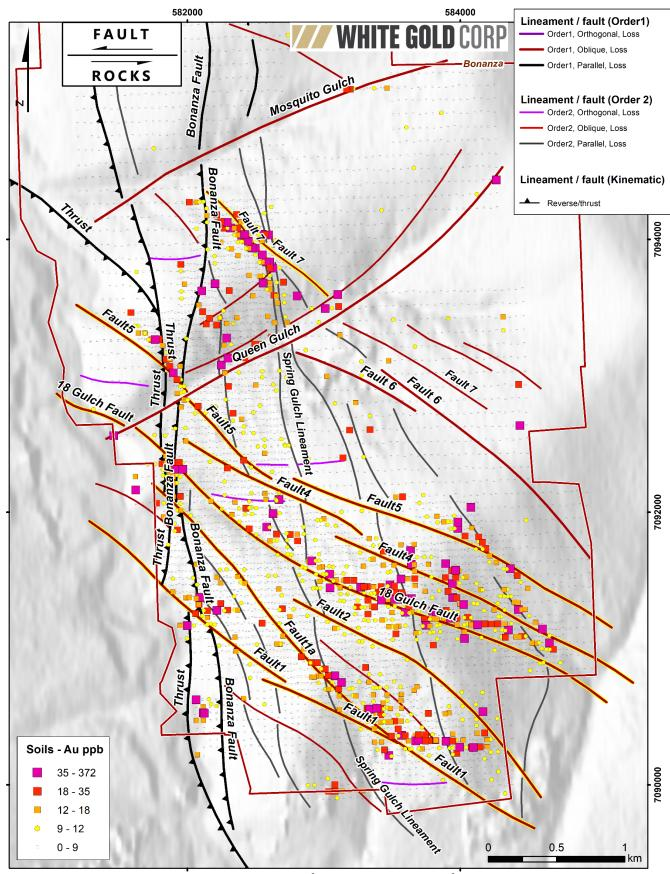
Figure 6: Interpreted Structures (Fault Rocks Inc.) and Gold in Soils on Shaded Relief DEM Base Map.
