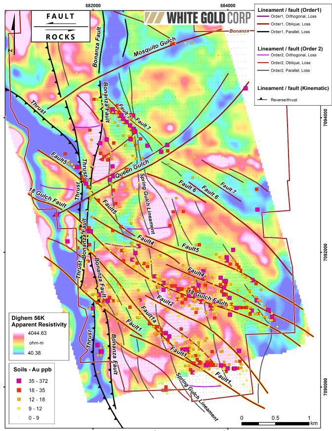
Figure 4: Interpreted Structures (Fault Rocks Inc.) and Gold in Soils on Airborne Dighem Resistivity 56K Base Map.
